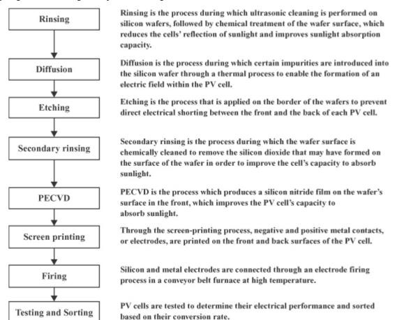
The following diagram shows the production procedures for our PV modules:
